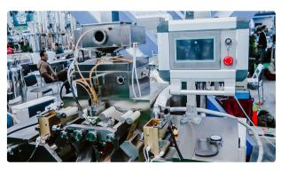
Pharmaceutical equipment for the production of soft gel gelatin capsules with oil inside
