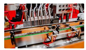
Automatic equipment for filling liquid products in glass bottles
