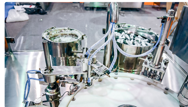
Automatic equipment for bottling and capping plastic bottles with spray nozzle
