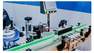
Automatic labeling machine for sticking selfadhesive labels on glass bottles with syrup Pharmaceutical Packaging • 22.09.2020 • 18.740K views
