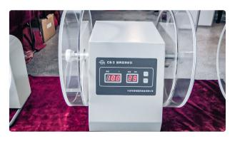
Automatic equipment for testing the abrasion rate of tablets and capsules in pharmaceutical...
