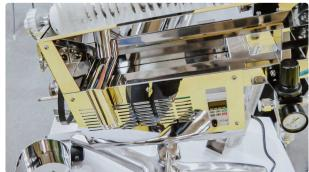
Pharmaceutical equipment for polishing hard gelatin capsules and dust removal
