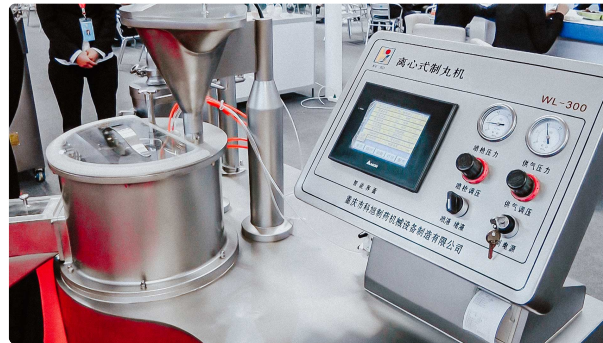
Automatic granulation and production machine for round spherical pellets Pharmaceutical Packaging • 17.09.2020 • 10.045K views
