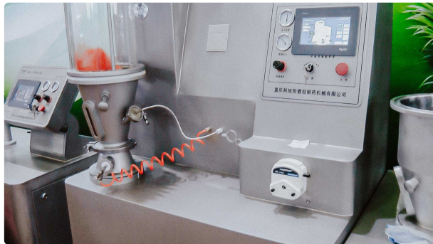
Laboratory equipment for drying and granulation in fluidized bed for pellet production Pharmaceutical Packaging • 14.09.2020 • 1.455K views
