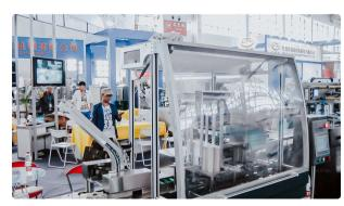
Automatic cartoning machine for packing blisters and plastic tubes into boxes CANADA
