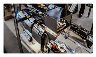
Automatic mill for production of fine powder fraction for pharmaceutical and food use
