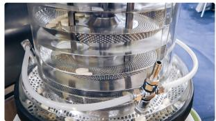
Automatic equipment for tablet polishing and dust removal in pharmaceutical production...
