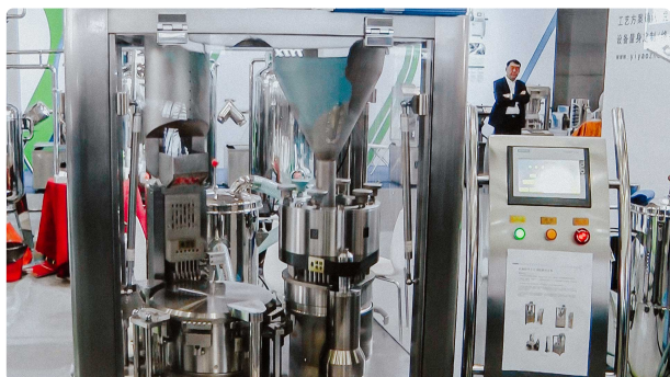
Equipment filling solid gelatin capsules with drug powder
