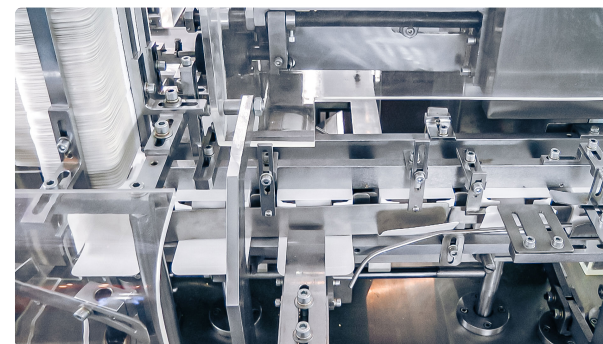
Automatic packaging equipment sachet in boxes in pharmaceutical production
