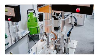
Desktop semi-automatic machine for screwing caps on plastic bottles
