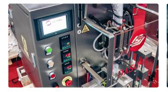
Equipment for packing in plastic bags of powder products and pellets
