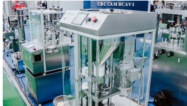
Automatic tablet press one punch for pressing tablets in the laboratory
