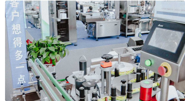
Automatic labeling equipment for double labeling of self-adhesive labels on bottles
