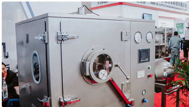
Automatic coater for tablet protective coating Pharmaceutical Tablet Press • 09.09.2020 • 2.890K views
