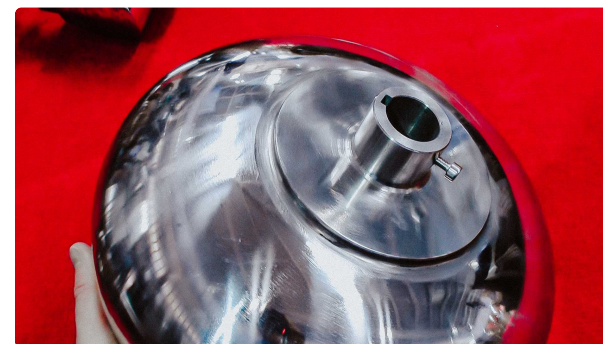
Coater for applying the tablet shell for pharmaceutical laboratory drug manufacturing
