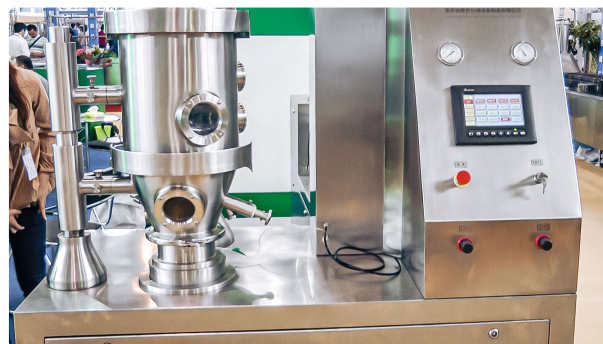
Automatic equipment for drying and granulation of powder in fluidized bed...
