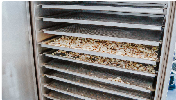
Special drying box with stainless steel shelves for product drying
