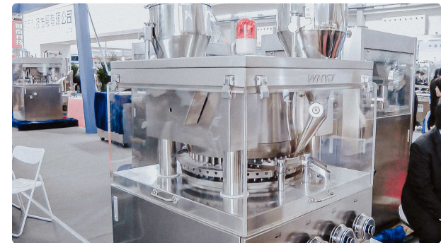
High speed automatic rotary tablet press for pharmaceutical tablet pressing USA
