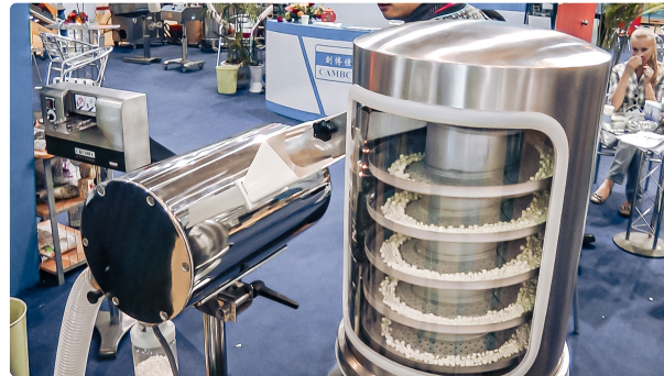
Automatic equipment for dedusting and polishing of tablets in pharmaceutical...
