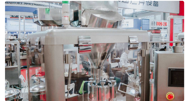
Automatic filling machine for solid gelatine capsules 00,0,1,2,3,4 with powder or granules
