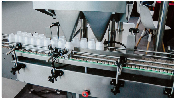
Line automatic filling and counting machine for tablet in plastic bottles
