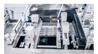
Automatic equipment for packing penicillin vials into plastic blisters in pharmaceutical...
