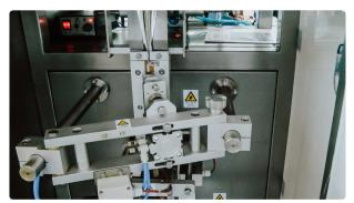
Automatic filling machine for dosing powder into packaging plastic stick bags
