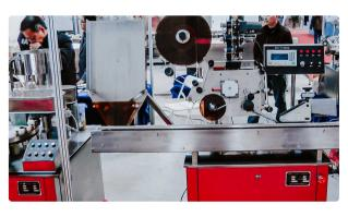
Equipment for self-adhesive labels on glass ampoules
