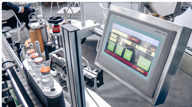
Automatic equipment for sticking self-adhesive labels on penicillin vials for pharmaceutical...
