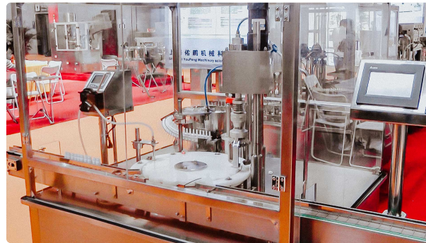
Mono block for filling and capping spray nozzle for plastic bottles
