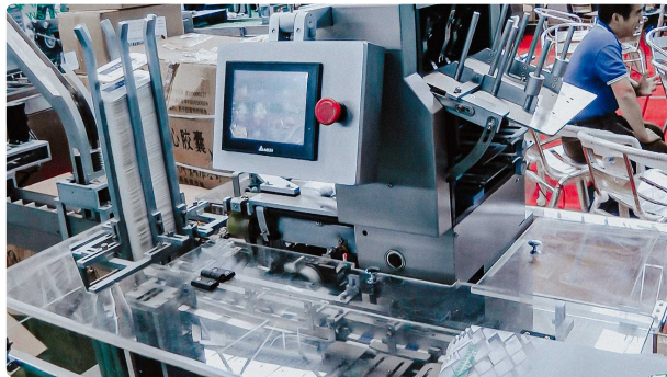
Pharmaceutical cartoning equipment to package the drugs in cardboard boxes
