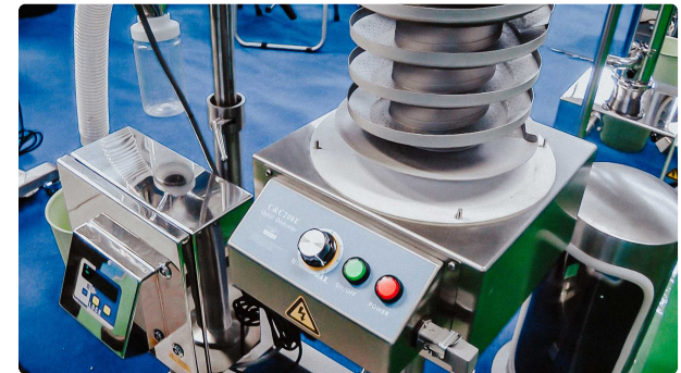
Automatic vibrating tablet lifting machine with automatic quality control in metal detector
