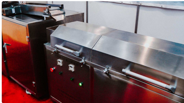
Drum dryers for soft gelatin capsules pharmaceutical production line
