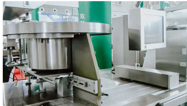
High speed automatic blister machine for tablet packaging in PVC and ALU blisters
