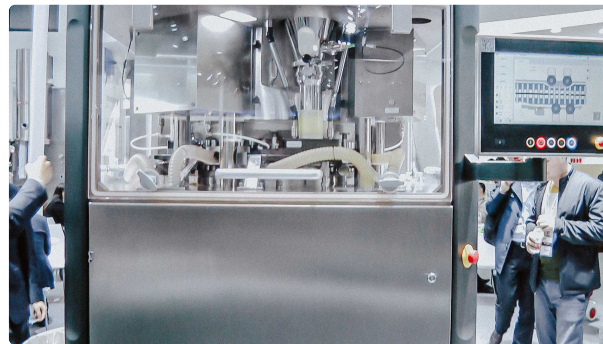
High quality rotary tablet press with dust collection system for tablets
