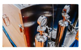
Equipment for washing and sterilizing glass bottles in the production of medicines
