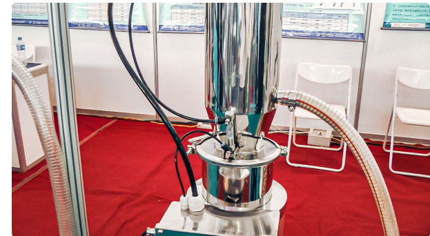
Automatic equipment for vacuum transport of powder in pharmaceutical production
