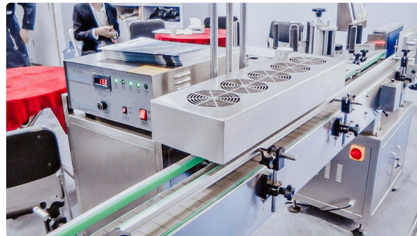
Automatic feed and put cap on plastic capping bottles
