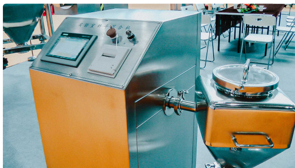
Cone mixer for mixing powders in pharmaceutical production of medicines
