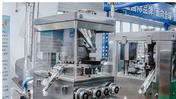
High speed automatic rotary tablet press for pharmaceutical tablet pressing
