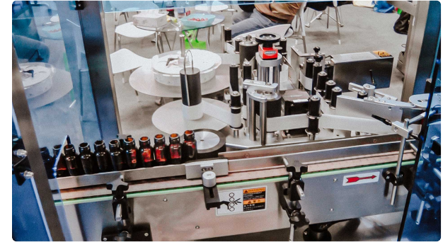
Automatic labeling machine for labelling labels on glass bottles
