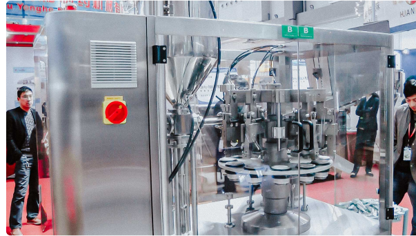
Pharmaceutical equipment for filling and sealing plastic tubes with cream and ointment
