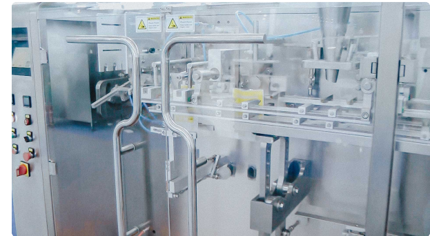
Automatic filling machine for dosing powders and granules into sachet bags
