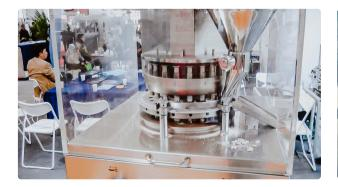
Automatic tablet making machine for pharmaceutical factory
