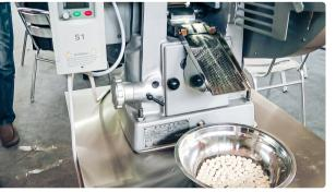
Automatic equipment for pressing laboratory tablets in pharmaceutical production
