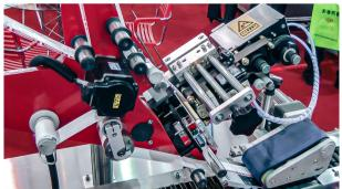
Automatic equipment to stick self-adhesive labels on penicillin vials in pharmaceutical...
