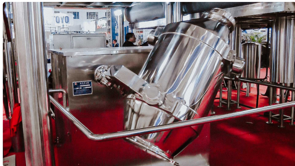
Powder mixing drum for pharmaceutical production
