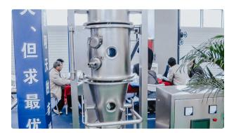
Automated equipment for drying and granulating of the powder in a fluidized bed
