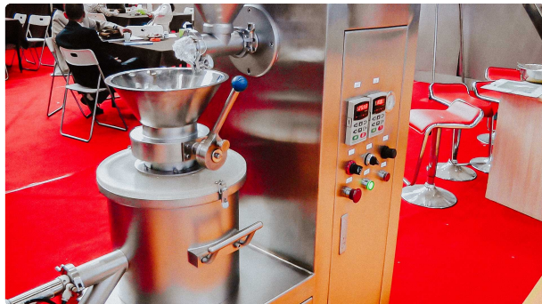
Granulator for pharmaceutical production of round shaped pellets medicine production
