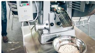
Automatic equipment for pressing laboratory tablets in pharmaceutical production
