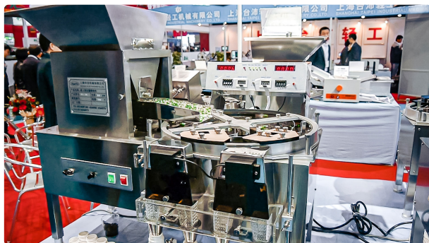
Automatic equipment for counting and packing of gelatin capsules into bottles Spain
