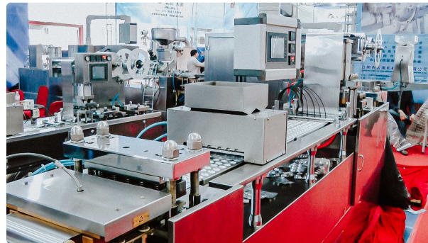
Automatic blistering machine for filling of tablets in blisters ALU / ALU
