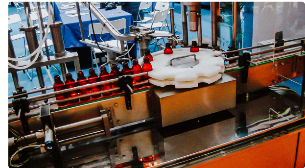
Automatic machine for bottling and capping plastic bottles plastic caps
