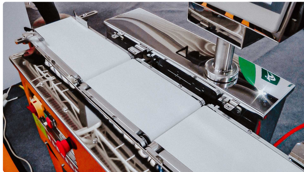
Conveyor scales for controlling the weight of drug packages in pharmaceutical production
